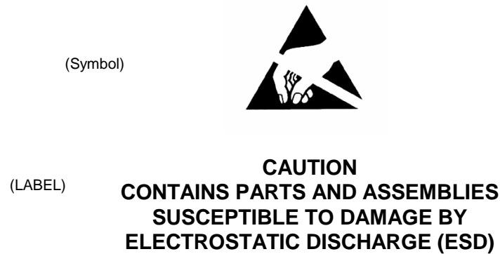
FIGURE 17. Electrostatic discharge (ESD) sensitive identification.
