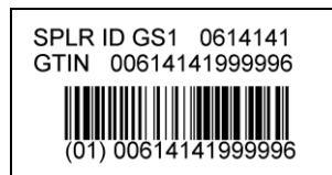
FIGURE 13. Example of GS1 System label (non-UID) for a part.
